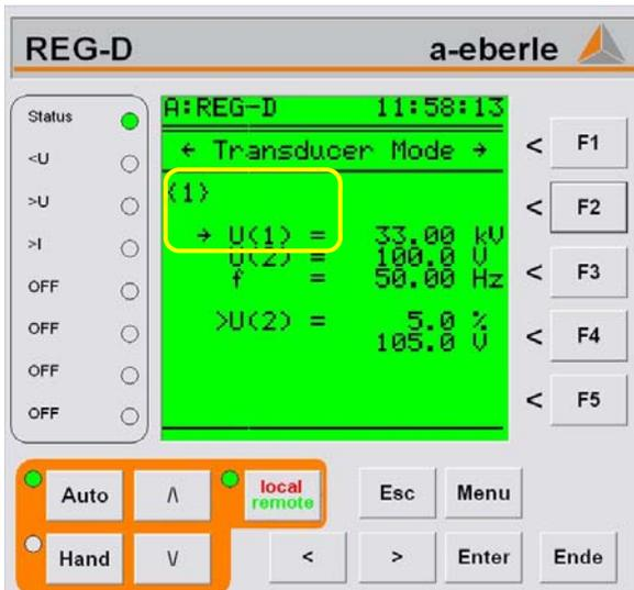
In the transducer mode you can see both voltages, the frequency and the supervision limit for the unregulated voltage.
