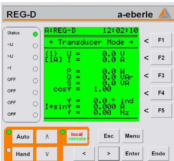
On the second transducer screen you can find the current, phase angle and the power of the regulated measurement input.
