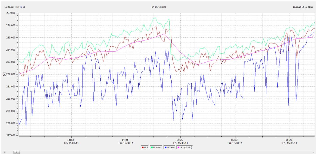
**Figure 2. Example 10 ms Max/Min, 60 second and 10 minute voltage data.**
