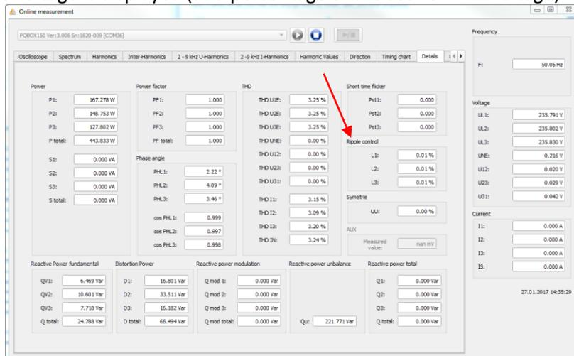
**Figure 5. Online measurement – instantaneous ripple voltage.**
