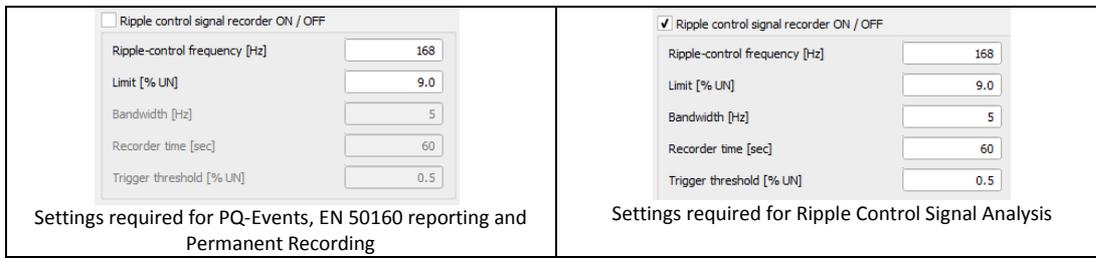
**Figure 1. Ripple control signal setup.**
