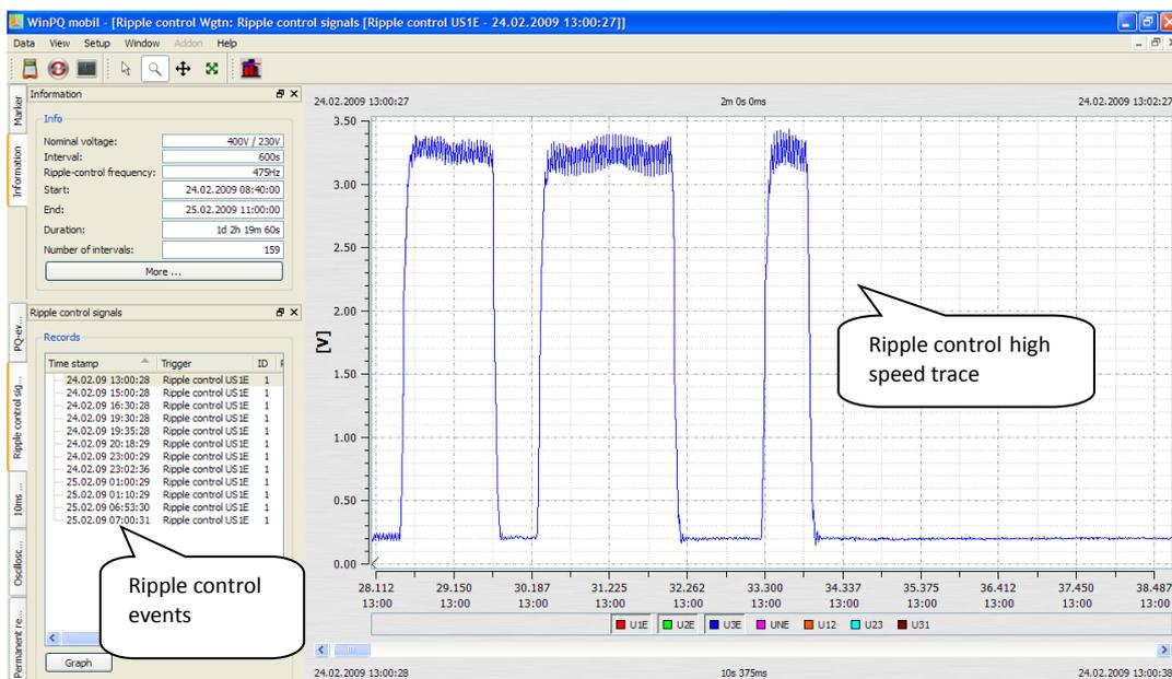
**Figure 6. Example high speed ripple control signal data (10 ms resolution).**
