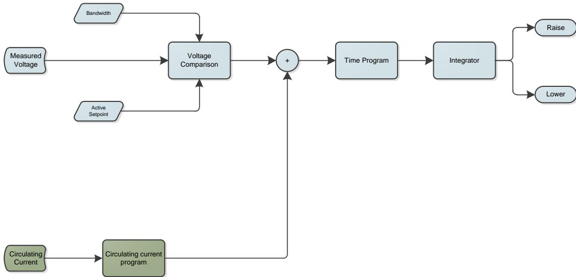
**Figure 5. The voltage regulation logic with the additional influence of circulating current.**
