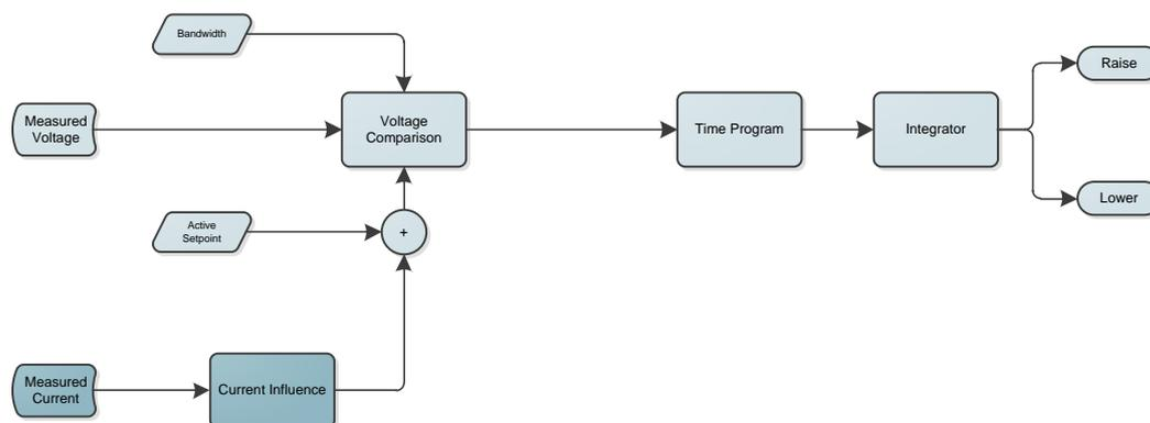
**Figure 2. Basic behaviour with Current Influence applied.**
