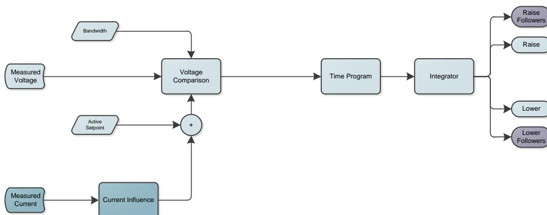
**Figure 4. Master-Follower scheme modified with the addition of a Current Influence program.**
