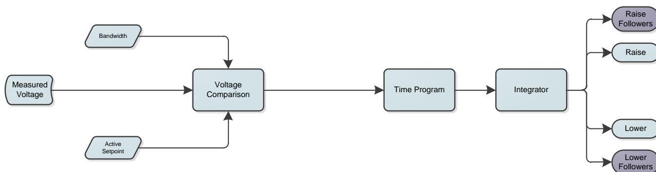
**Figure 3. Master-Follower scheme (Master relay logic shown). The Master makes tapping decisions which are mimicked by 'Following' relays.**
