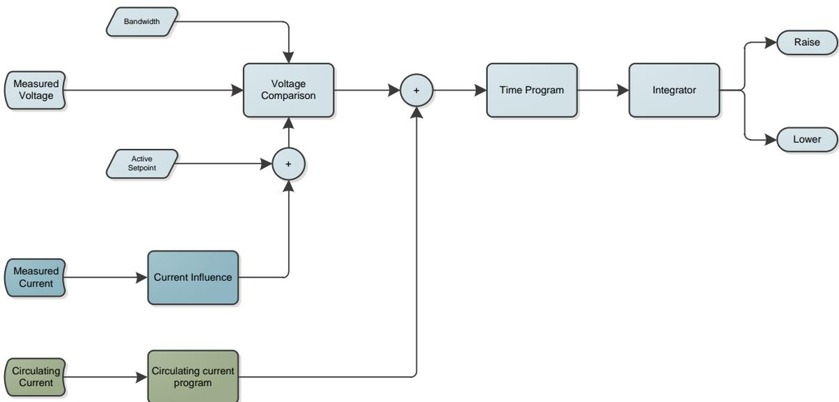
**Figure 6. Circulating-Current parallel scheme with Current Influence applied.**
