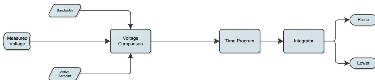
**Figure 1. The basic voltage regulation function of a VRR (without any Current Influence or parallel programs).**
