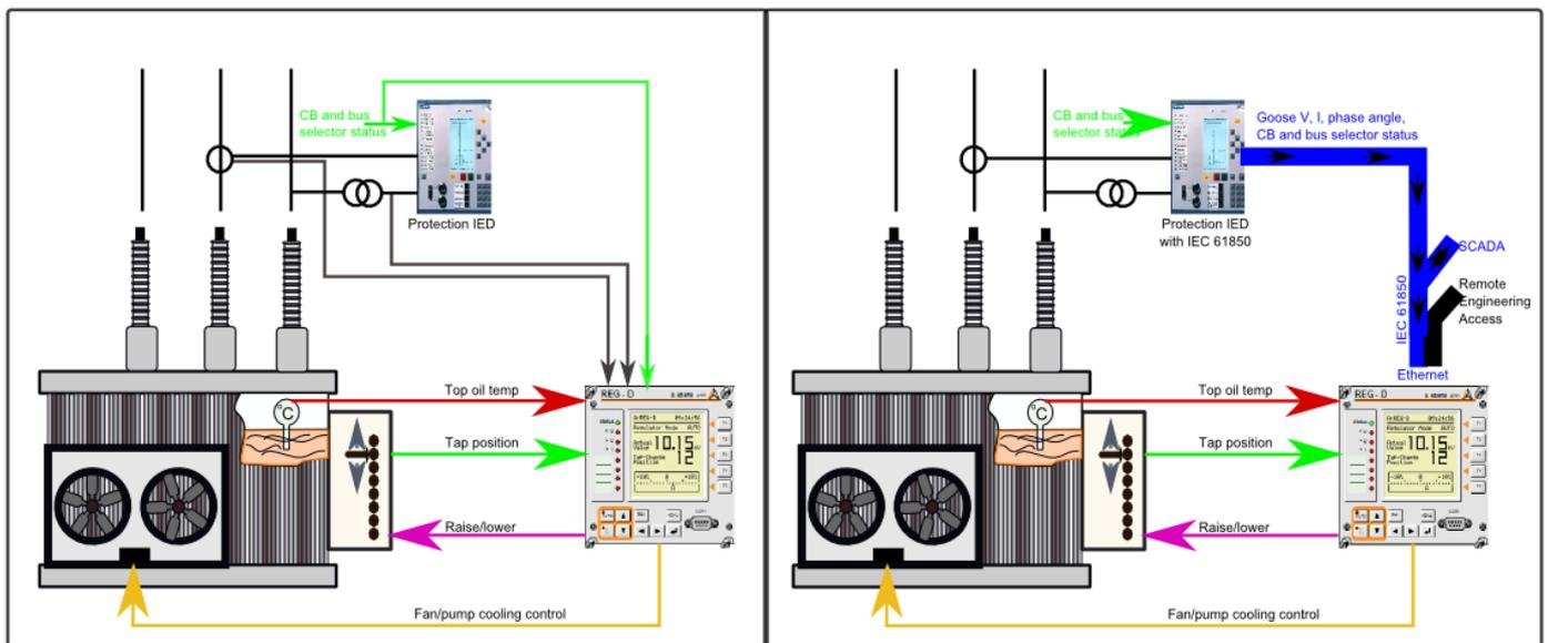
**Figure 2. GOOSE messaging (right) replacing hardwire current/voltage inputs (left)**
