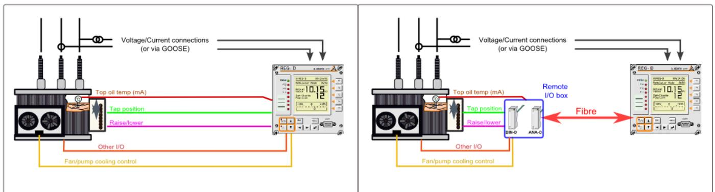
**Figure 1. Traditional Voltage Regulator Relay Connection (left) & remote I/O box marshalling at transformer (right)**
