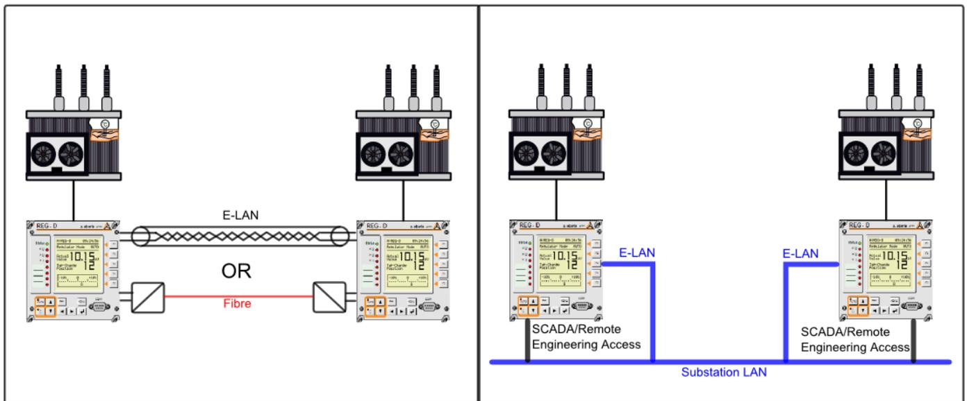
**Figure 3. E-LAN communication via traditional E-LAN (left) and Ethernet (right)**
