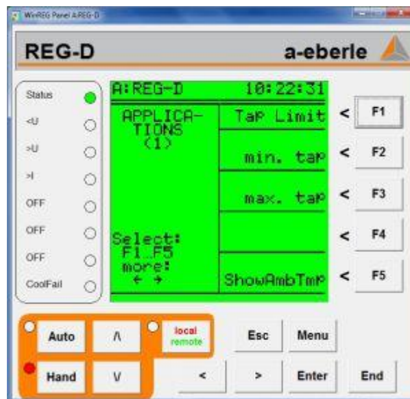
Figure 3. Example of REG-D customised screen for user defined settings, which can be developed using H-Code.
