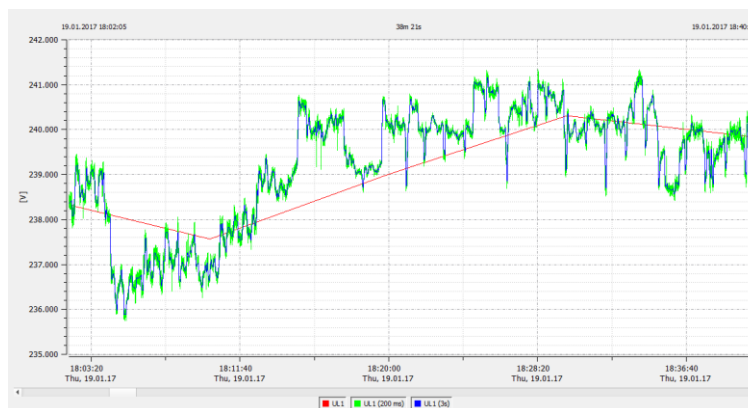
Figure 11. Example of voltage trace with 200 ms, 3 s and 10 minute data class.
