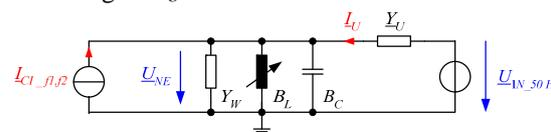
Fig. 1: Simple equivalent circuit with current injection
