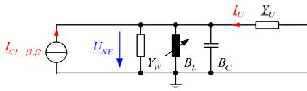
Fig. 2: Simple equivalent circuit with current injection unequal to 50 Hz
