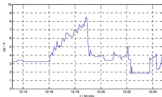
Fig. 9: Disturbed  $U_0$  without switch-operation or coil movement
