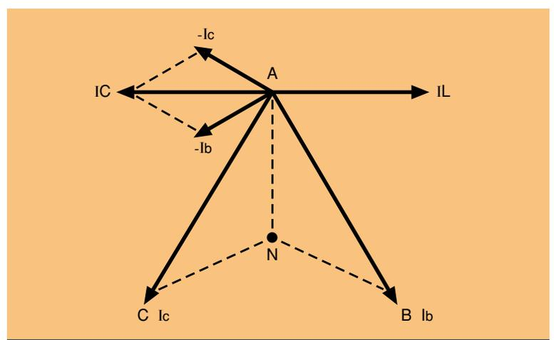
Fig. 1a: Current vectors for A phase fault
