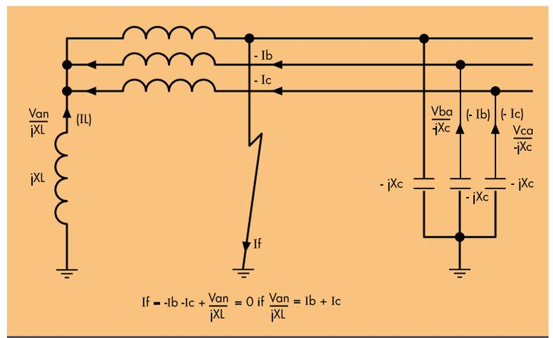
Fig. 1: Current distribution in Petersen Coil earthed system
