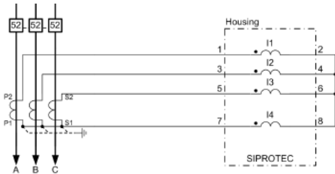
7UT85 Current Transformer connection: 3- phase + IN
