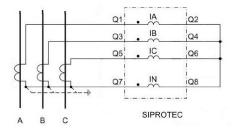
In a line protection relay the possible options are that the CT star-point is towards the line or towards the busbar. In a 7UT relay the options are that the star-point is towards the protected object (eg. transformer) or not towards the protected object. This can easily be seen from the drawings and applied as a relay setting.
