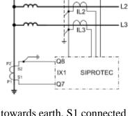
P1 towards earth, S1 connected to Q7. Set 0711 'EARTH iX1 AT' = Q7
