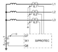
P2 towards earth, S2 connected to Q8. Set 'EARTH iX1 AT' = Q8
