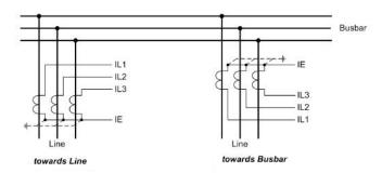
If the CT secondary star-point connection is to the correct relay terminals then the CT primary orientation can be either way without affect on the relay. This is shown in the following two examples - a fault towards the line results in the same secondary currents into the relay, even though the CT primary orientation has been swapped.
