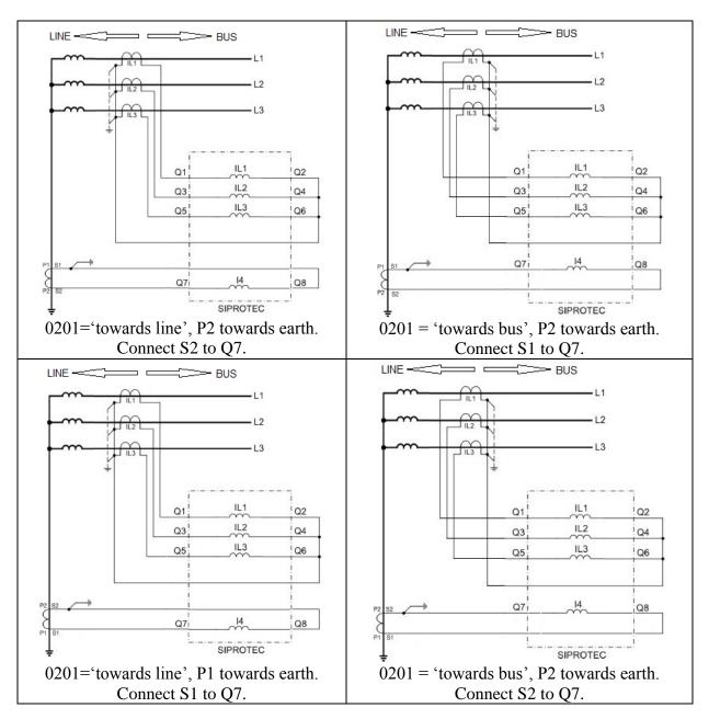
The secondary earthing of the CT is required but its location is not relevant to the setting.
