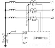
P2 towards earth, S2 connected to Q7. Set 'EARTH iX1 AT' = Q7
