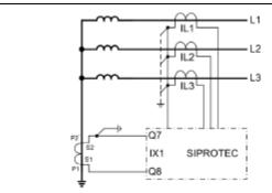
P1 towards earth, S1 connected to Q8. Set 0711 'EARTH iX1 AT' = Q8
