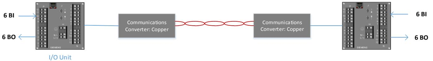
**Figure 4. Binary signal transfer using a pair of 7XV5673 I/O units**
