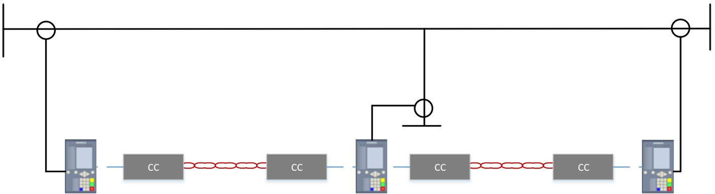
**Figure 3. Three-terminal line differential using 2 pilot wires**
