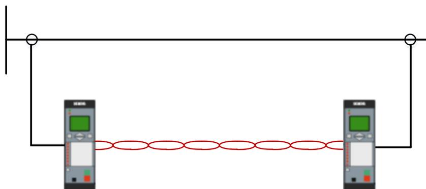
**Figure 1. Differential protection of a two-terminal line using 7SD80 relays connected directly to pilot wire**
