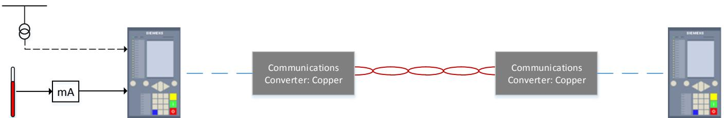
**Figure 6. Transfer of user-defined analogue signals between substations.**
