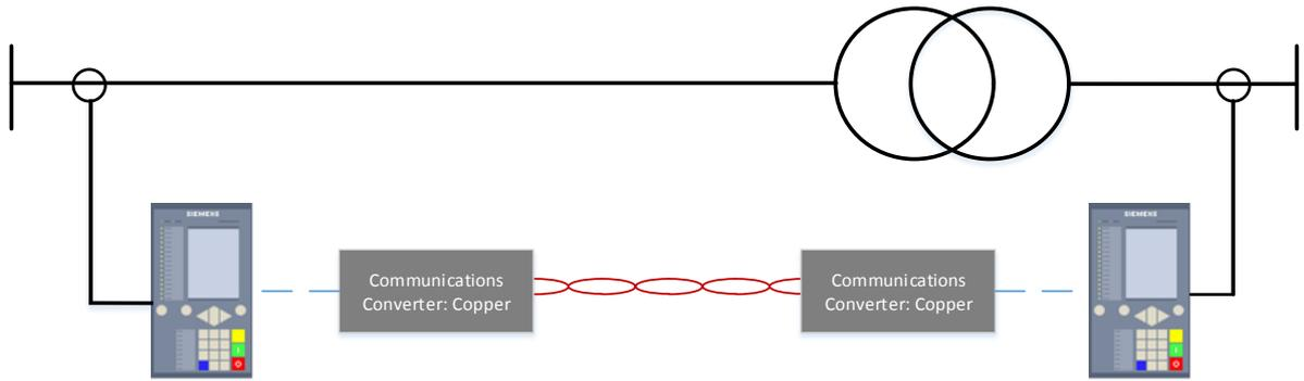
**Figure 2. Line differential with transformer-in-zone using SIPROTEC 5 relays with communication converters for pilot wire**
