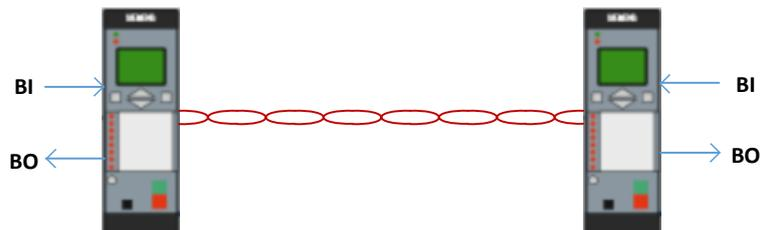
**Figure 5. Binary signal transfer using 7SD80 relays directly connected to pilot wire.**
