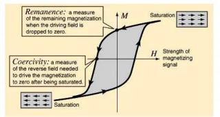
Figure 2: B-H Magnetizing Curve for any magnetic material
