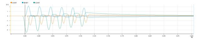
Figure 5: Typical transformer inrush current asymmetric waveform.
