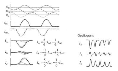
Figure 4: Origin of three phase magnetizing current waveforms with theoretical quantification.
