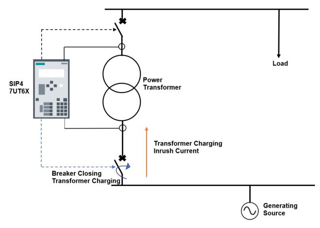
Figure 1: Schematic diagram of switching on an unloaded power transformer
