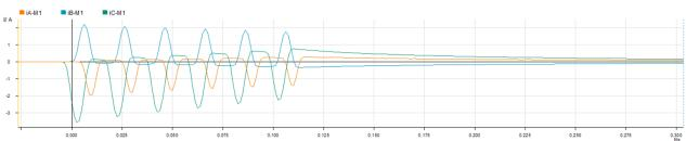
Figure 9: Current Waveform injected to the 7UT613 recorded in SIGRA
