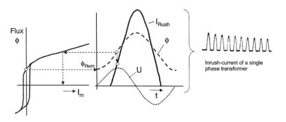
Figure 3: Origin of single phase magnetizing current waveform.
