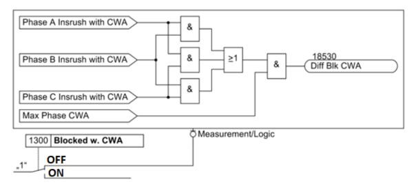
Figure 6: Logic for Current Waveform Analysis Restraint (CWA)
