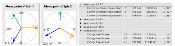
Figure 14: Analog Inputs of Special Treatment with Protected Object GSUT
