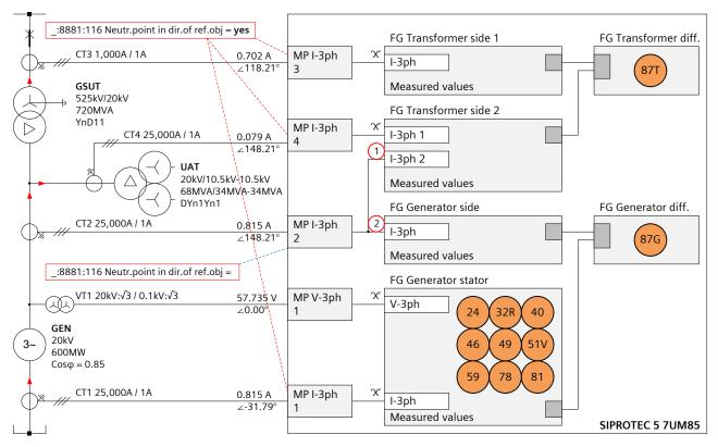
Figure 1: Conventional Connection Diagram for FG Generator Stator
