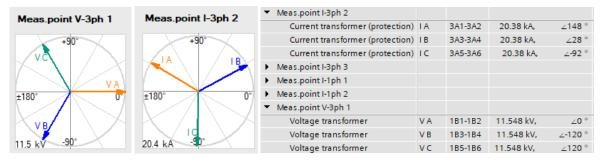
Figure 7: Measured Phasors with Protected Object GEN
