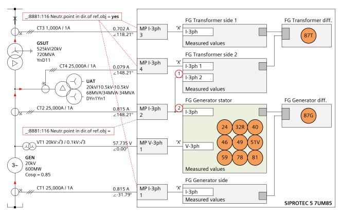
Figure 5: Connection Diagram with Lead Current for FG Generator Stator – Incorrect Solution
