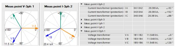
Figure 8: Measured Phasors with Protected Object GSUT
