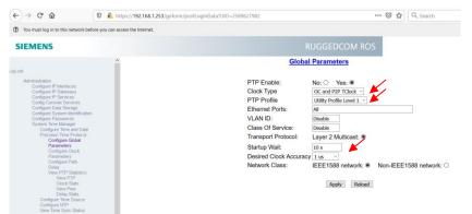
Figure 4: RSG909R PTP Global Parameters
