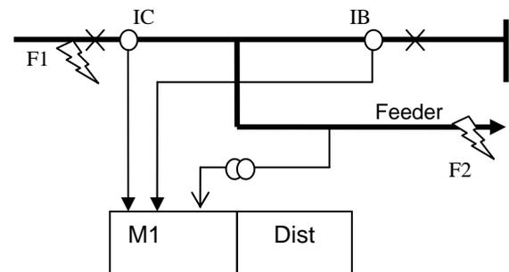
**Figure 8: Distance protection with separate measurement of both CT currents**
