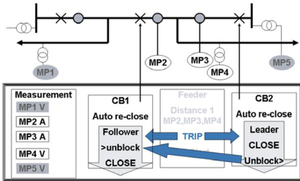
**Figure 16: Multiple AR functions with internal co-ordination**
