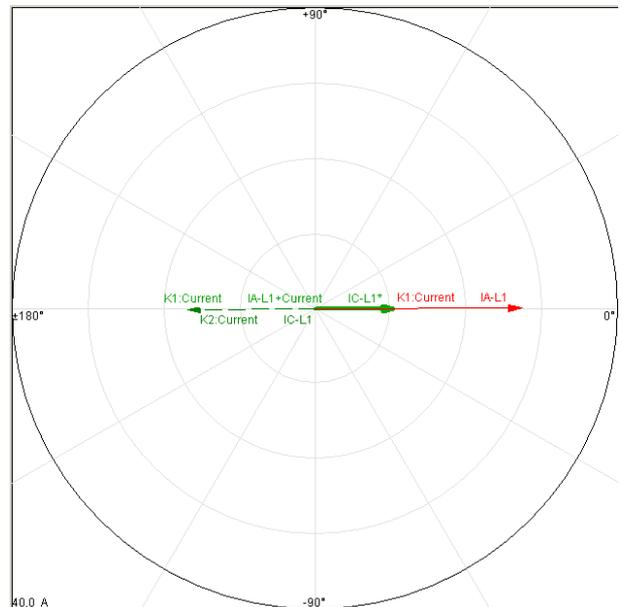
**Figure 13: Filtered fundamental component amplitude during remote forward fault (F2)**
