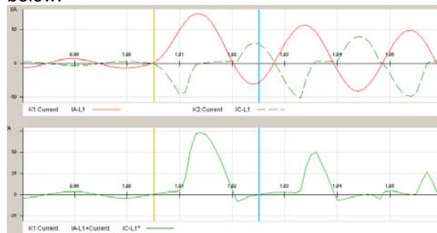
Figure 10: Current waveform during close in reverse fault (F1)
