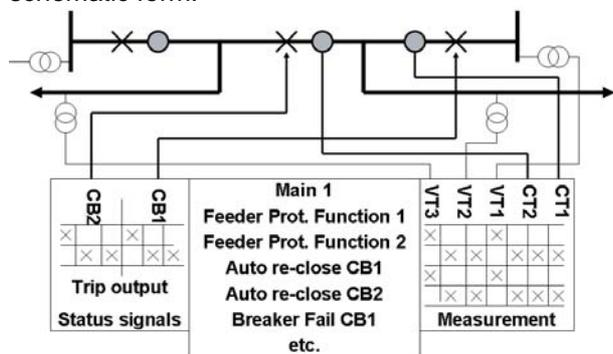
Figure 1: Connection of IED
