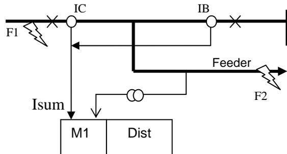
**Figure 7: Distance protection with external summation of both CT currents**
