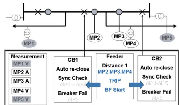
Figure 15: Assignment of measuring points and internal signal exchange
