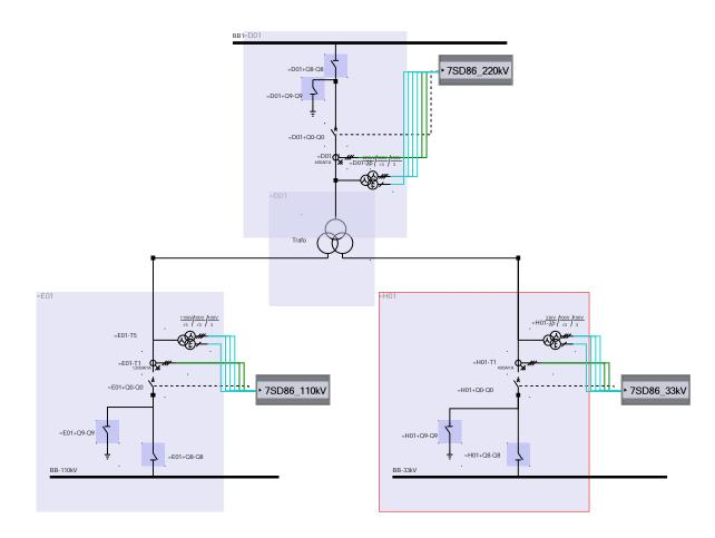
The selection of line differential protection due to the large distances and the derived settings taking a three-winding transformer as an example is described in this application.
