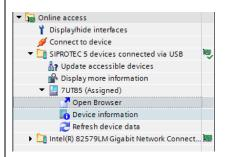
Note that it is actually possible to open the web browsers using the front panel USB connection. As DIGSI 5 uses an IP mechanism over the USB serial port to communicate securely with the relay – this also allows a browser connection. The IP address for the USB port can be found via the relay front panel menu [Test and diagnosis/IP-Configuration/Onboard USB].
