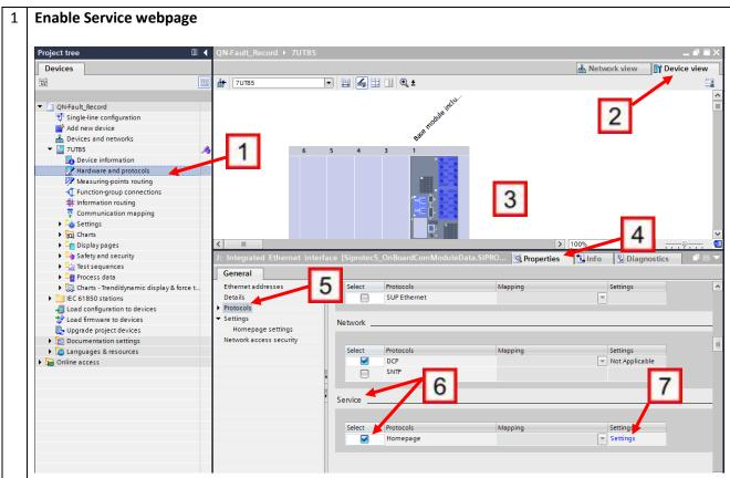
Via the Project Tree, select 1 "Hardware and Protocols", then 2, Device View Tab. 3, the Ethernet interface desired. 4, select Properties.
