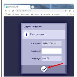
The above example does not have role based access enabled, so simply click the tick button for default user "SIPROTEC 5" access – no password is set as default.
