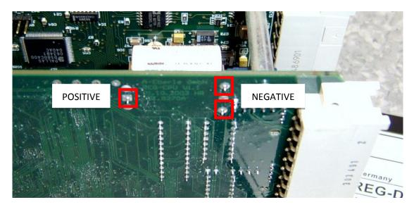
Carefully unsolder the battery from the board. Take note that there is one pin to be unsoldered on one side of the battery and *one or two* pins on the other side, as shown above.
