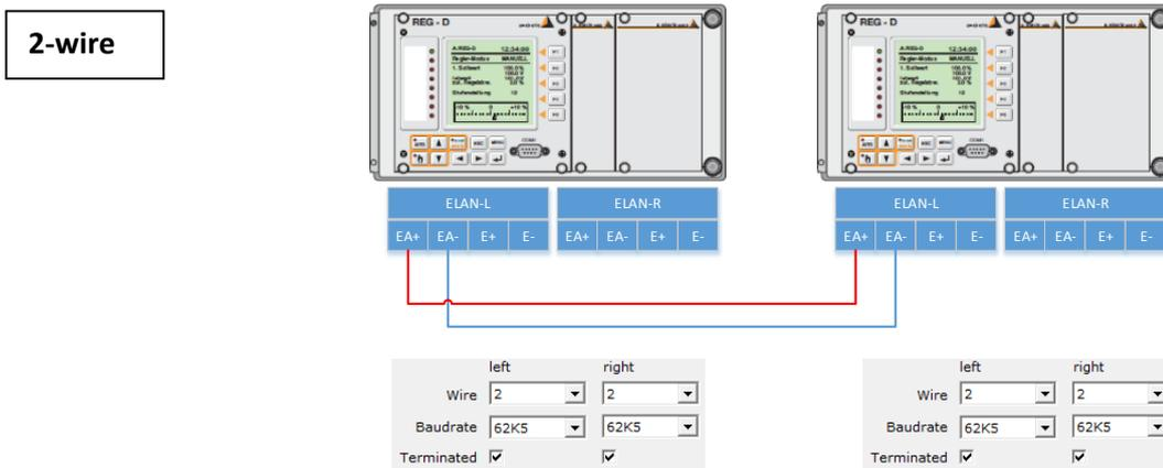
**Figure 9. An example of a 2-Wire E-LAN network for two relays. Only the left ports are use in this example. 'Terminated' is set ON for both relays.**
