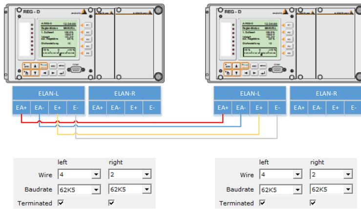
Figure 11. An example of a 4-Wire E-LAN network for two relays.
