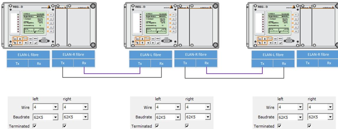
Figure 13. An example of an E-LAN via fibre. The connection parameters are the same as those for the 4-wire connection method.
