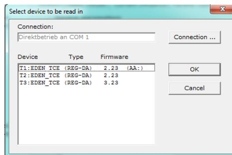
Figure 8. Selection of the device on the E-LAN network to connect to via WinREG. The relay that the computer is directly connected to is indicated by (AA:). Connection to the other devices would be via E-LAN.
