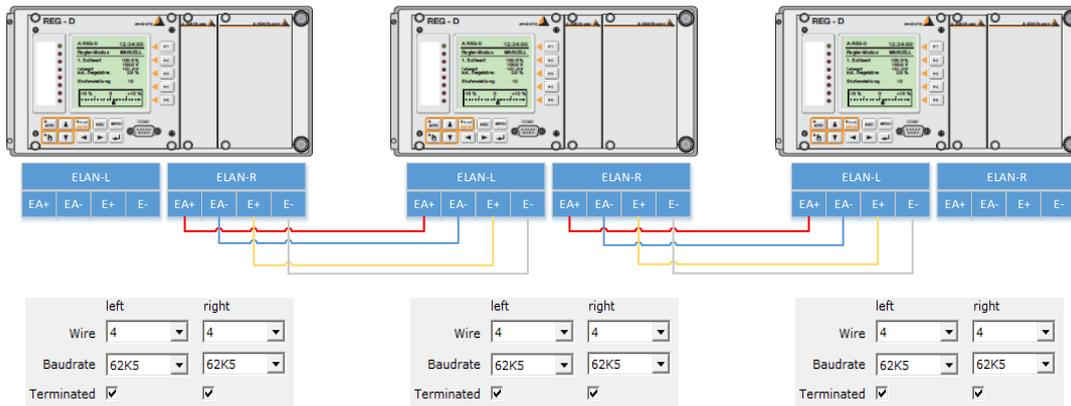
Figure 12. An example of a 4-Wire E-LAN network for three relays. Each link is a point-point connection so both E-LAN ports are used on the centre device.
