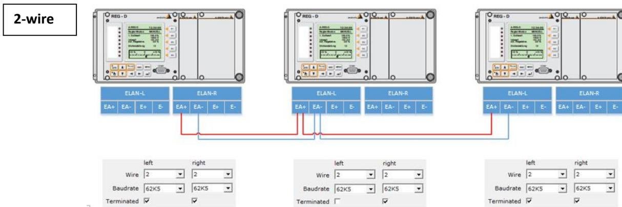
**Figure 10. An example of a 2-Wire E-LAN network for three relays. The 'Termination' setting is ON at the two devices at the end of the bus and OFF on the centre device.**
