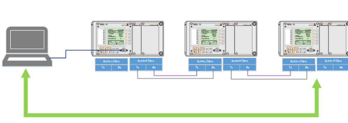
**Figure 1. An E-LAN network using multiple point-to-point links. The laptop connected to the front-port of the relay at the left can use the E-LAN to connect WinREG to any of the relays.**
