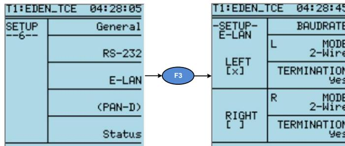
**Figure 5. The E-LAN setup and commissioning page is accessed via the Setup 6 menu. Here the [X] shown for the E-LAN LEFT port indicates that it is active.**
