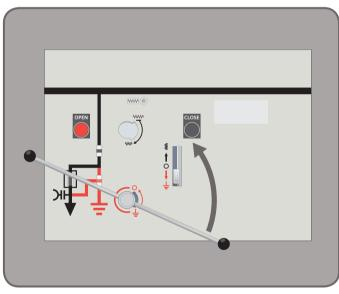
**2** Insert the Operating Lever and rotate anti-clockwise to open the Earth Switch.
