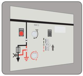
Remove the Operating Lever. Check the Control Gate has returned to the mid position.
