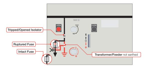
If a fuse ruptures, the Isolator will automatically open. The transformer/feeder circuit must be switched from Isolated to Earthed to allow the panel cover to be removed to facilitate fuse replacement (Step D, above).
