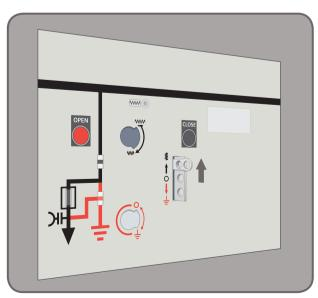
Slide the Control Gate up to open the Spring Charge Shutter.
