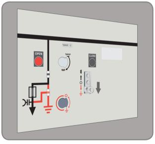
Slide the Control Gate down to open the Earth Shutter.
