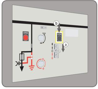
$\boldsymbol{3}$  (a) Remove the Operating Lever. Check the Control Gate has returned to the mid position.
