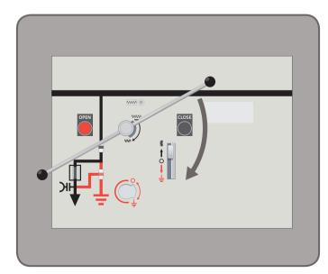
2 Insert the Operating Lever and rotate clockwise to charge the spring. It will click and hold when rotated enough (70°).
