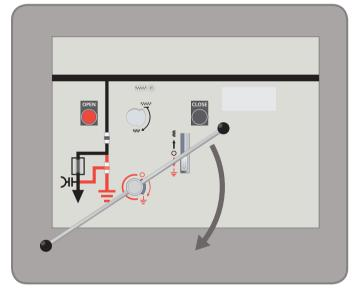
$\boldsymbol{2}$  Insert the Operating Lever and rotate clockwise to close the Earth Switch.
