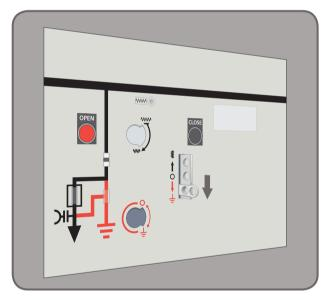
Slide the Control Gate down to open the Earth Shutter.
