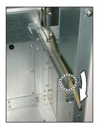
Fig. 531: Pushing the handle downwards to end position
