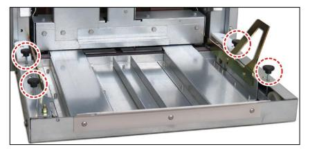
Fig. 449: Adjusting the height with the bolts
