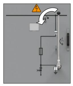
Fig. 415: Turning the operating lever counter-clockwise
