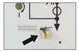
Fig. 294: Moving the lever to the left
