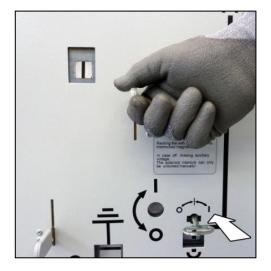
Fig. 290: Double-bit key inserted
