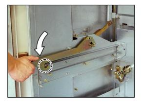
Fig. 526: Pushing the handle downwards to end position
