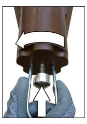
Fig. 475: Type 3: Unscrewing the contact cap
