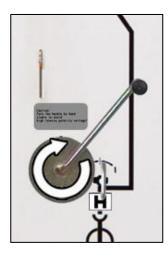
Fig. 716: Turning the racking crank clockwise
