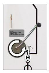
Fig. 720: Turning the racking crank counter-clockwise
