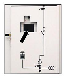
Fig. 733: Circuit-breaker type 3AE1: Inspection window for circuit-breaker position and closing spring state in control door
