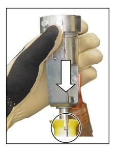
Fig. 680: Plug on tulip onto earthing rod
