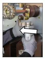
Fig. 176: Pushing the upper end into the clamp
