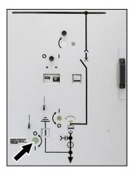
Fig. 101: Actuating opening on high-voltage door
