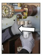
Fig. 373: Pushing the upper end into the clamp
