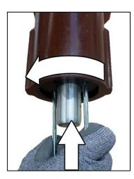
Fig. 476: Type 4: Unscrewing the contact cap
