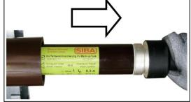
Fig. 471: Loosening fuse-link
