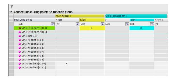
It is also important to notice that the trips released by every function group will act only on the corresponding circuit breaker per the configuration in DIGSI 5, that is control and protection from bays and circuit breakers completely independent from each other.
