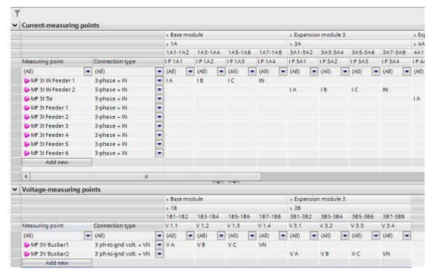
When all the measurement points have been properly created it is possible to assign each of them to the corresponding function group(s) to execute the related protection and control functionality. In the graphic below is shown, for example, that the 3-Phase current measuring coming from the In Feeder 1 is assigned to
