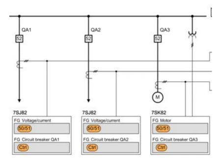
The new generation of protection and control devices SIPROTEC 5 allows protecting and controlling the complete switchgear (up to 9 bays) with a single device. In such a way is reduced not only the investment but also the parameterization and commissioning times.
