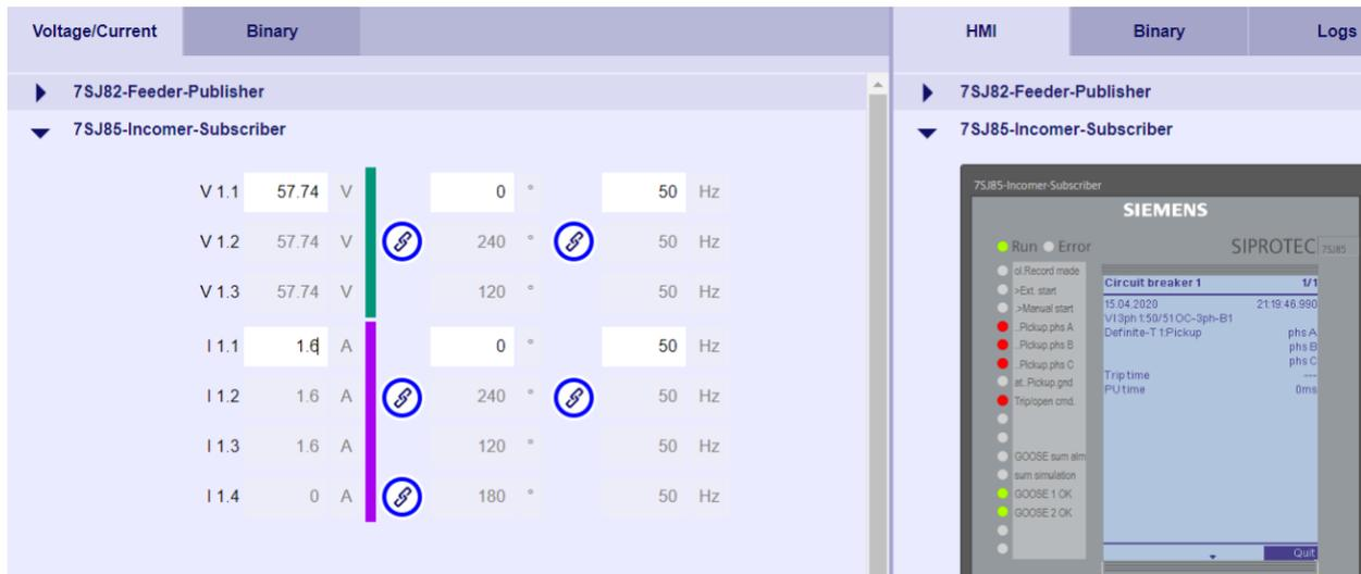
In this example, the secondary current was raised to 1.6A, which should lead to a triggering. As can be seen in the display of the protection device, all three phases respond, and the trigger command was passed on to the circuit breaker.
