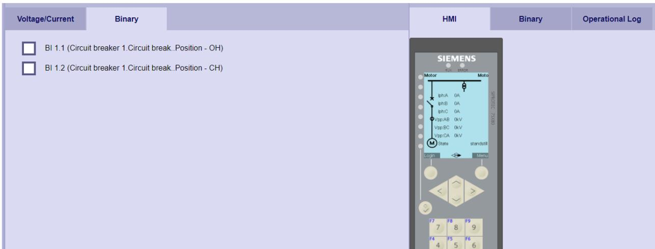
The same designations are displayed as on the front display. Either the full hierarchical or the alternative terms. The suffixes OH (open), CH (closed), H (high) or L (low) are automatically inserted according to the information ranking of the DIGSI 5 project. The states of the last simulation are preset.
