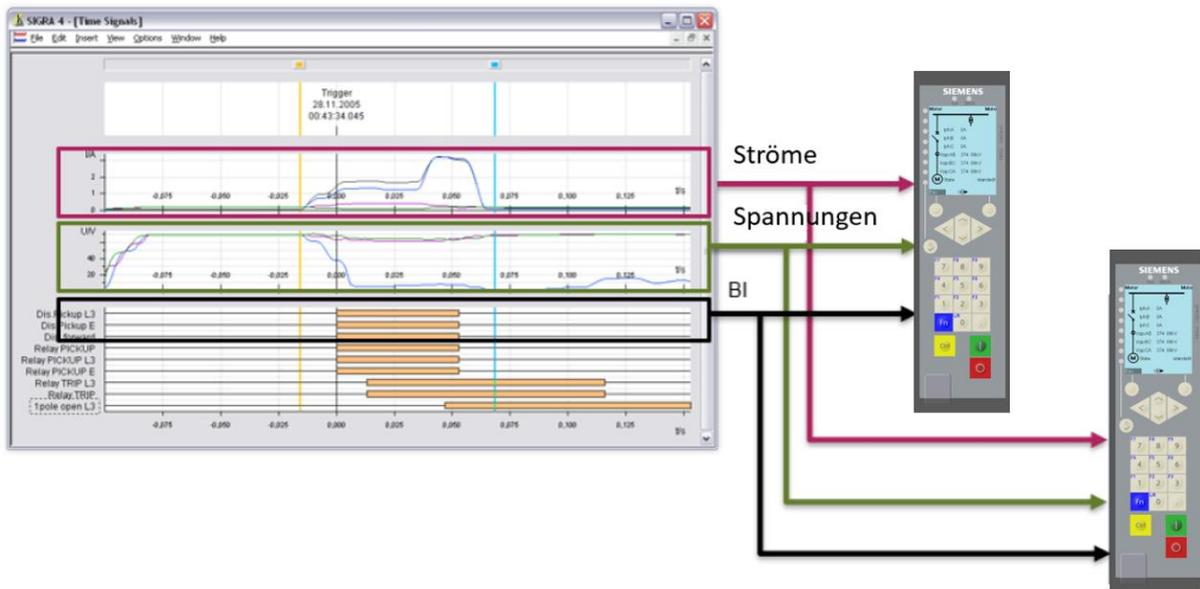
Upload your standard COMTRADE files (according to IEEE C37.111/ IEC 60255-24), with either primary or secondary values from the following sources:
