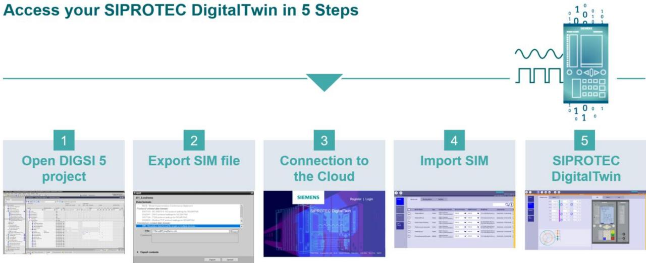
In general, either a single device or several devices from DIGSI 5 can be exported with the SIM data format and imported into SIPROTEC DigitalTwin.
