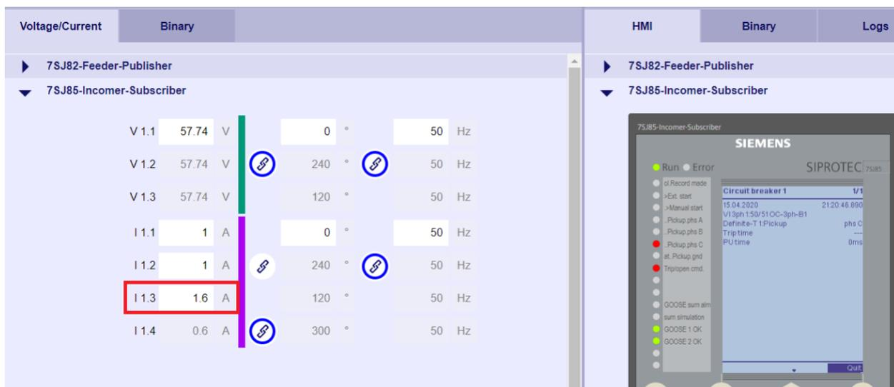
Analogously, the single-phase triggering can be tested. Here only the current of L3 was raised. This was also detected by the device which tripped accordingly.
