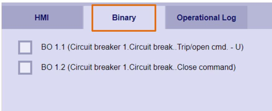
The labeling of the binary outputs is done in the same way as described in the previous chapter. In contrast to the binary inputs, the states cannot be changed here. The states are displayed as the contacts are controlled by the protection device.
