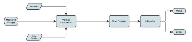
Figure 1. The basic voltage regulation function of a VRR (without any Current Influence or parallel programs).
