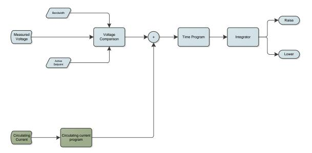
Figure 5. The voltage regulation logic with the additional influence of circulating current.
