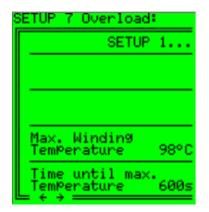
Max Winding Temp is like asking "at what temperature will my transformer be considered to be overloaded?" This is generally set to 98°C because this is the temp at which the transformer ages at normal time: 1hr = 1hr thermal ageing (Loss of Life)
