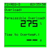
If the combination of load current and top oil temperature will result in a final winding temp of more than 98°C, the **Time to Overtemp** begins counting down to this event.
