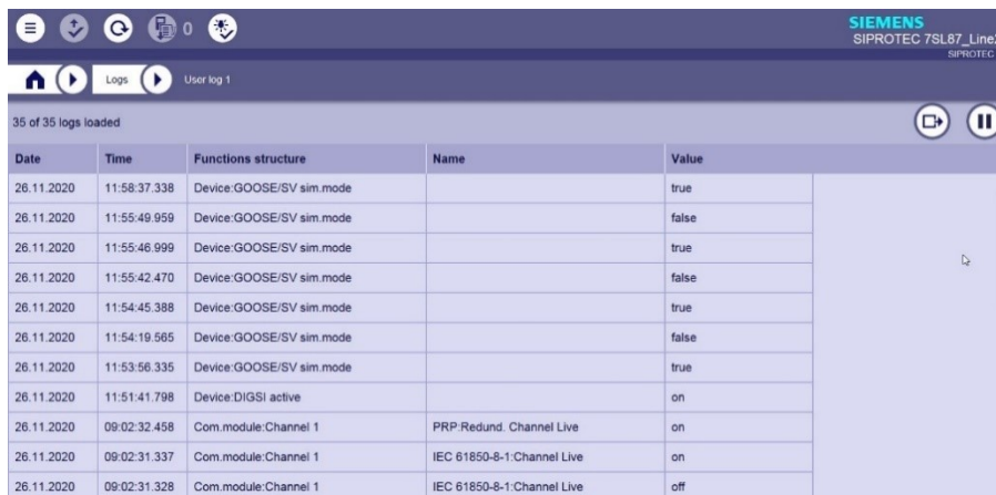
Figure 9. DIGSI 5 – IEC 61850 Simulation Status in Event Log
