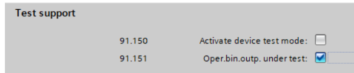
Figure 45. Test support menu in DIGSI 5 - recommended setting
