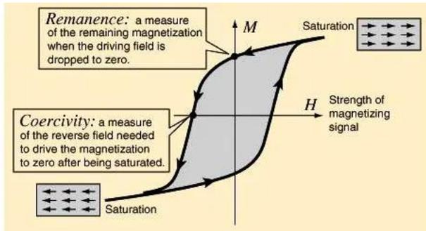
Figure 2: B-H Magnetizing Curve for any magnetic material
