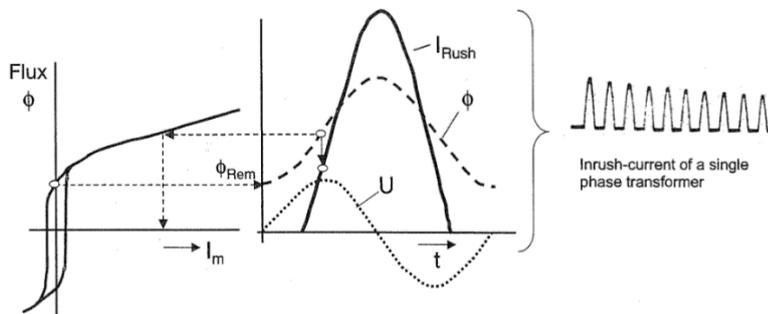
Figure 3: Origin of single phase magnetizing current waveform.
