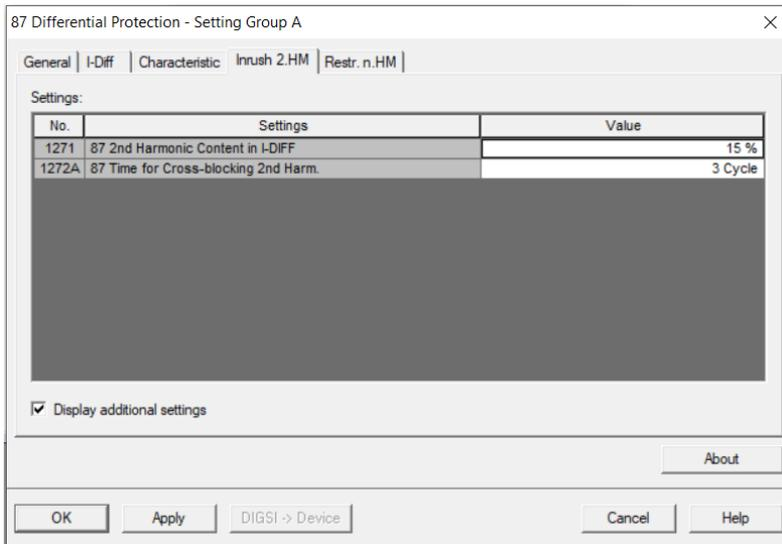
Figure 8: Setting parameterization for 2<sup>nd</sup> Harmonic Content in parallel with CWA.
