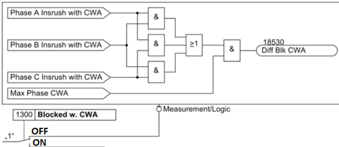
Figure 6: Logic for Current Waveform Analysis Restraint (CWA)
