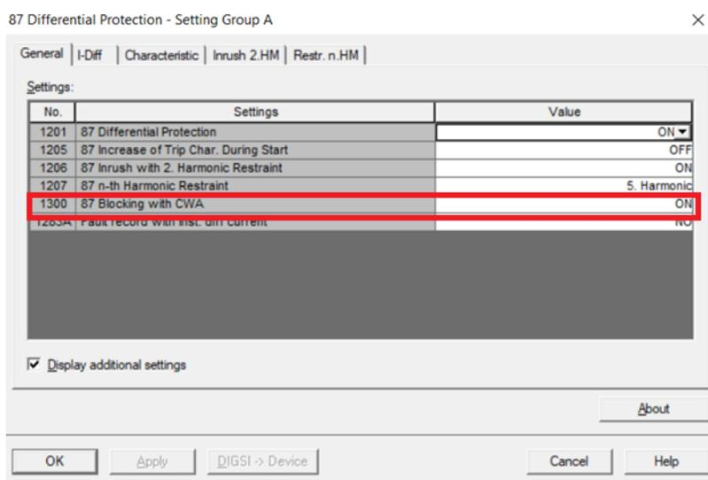
Figure 7: Setting parametrization required for CWA
