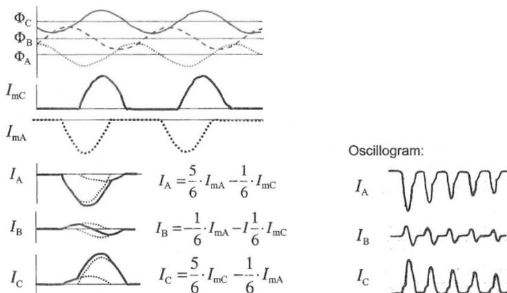
Figure 4: Origin of three phase magnetizing current waveforms with theoretical quantification.
