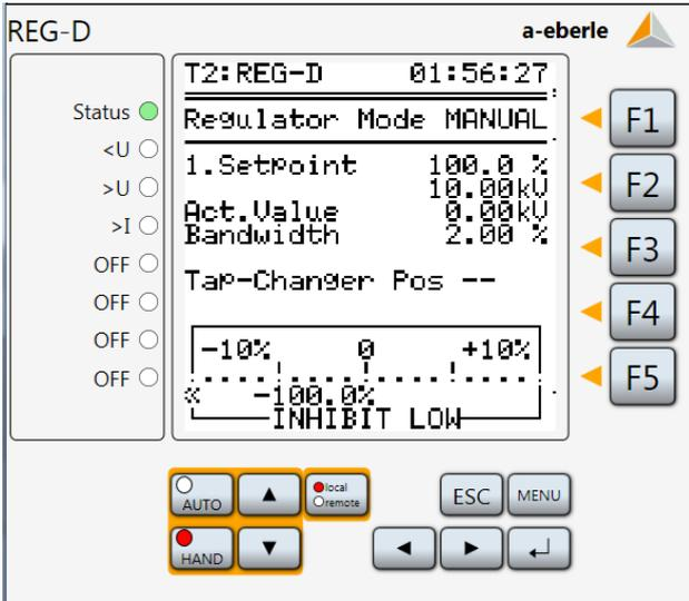
Press the Menu key, then the
