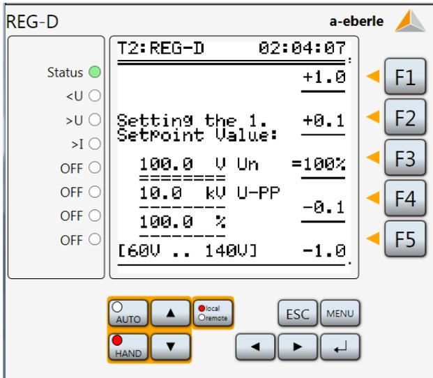
Use the F1, F2, F4 and F5 keys to set the setpoint to the required value. Note that the primary value is also shown below the secondary value to assist with this setting. In the example below, a setpoint of 11kV has been set:
