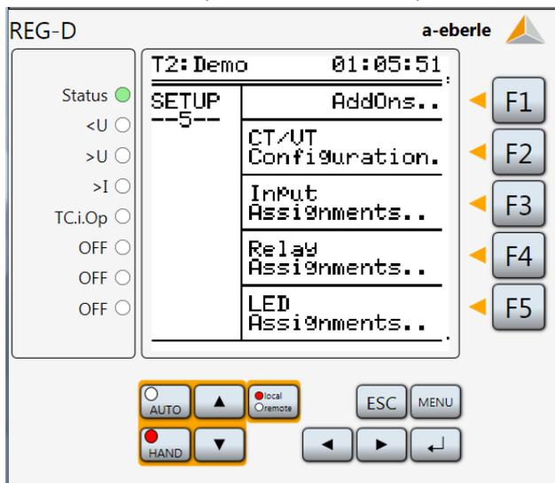
Next press the F2 key (CT/VT Configuration), so that the following display is shown:
