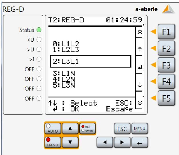
Once the correct setting is shown in the selection box, press the F3 or
