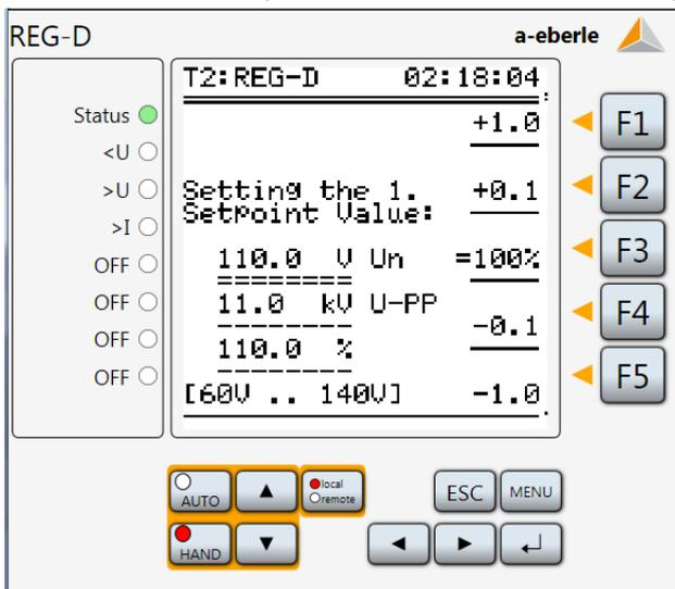
Once the required value has been reached, the F3 key should be pressed to bring the new value back to 100%.
