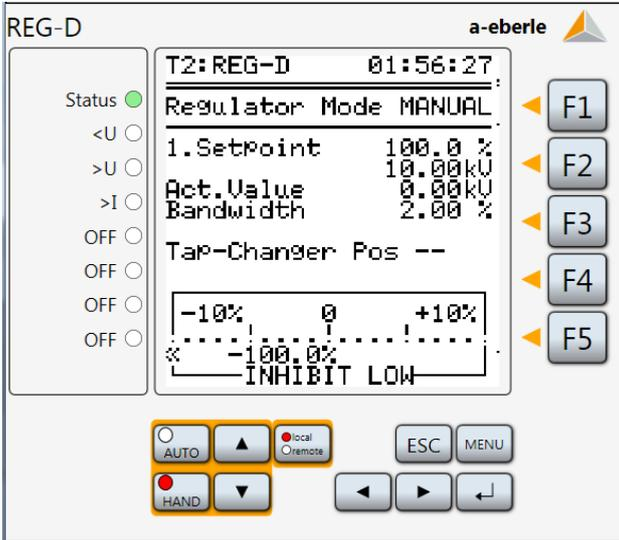
Press the Menu key 3 times, to access the Setup-1 menu, then press the F3 (Setpoint Values) key:
