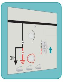
Remove the Operating Lever. Check the Control Gate has returned to the mid position.
