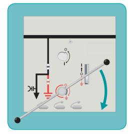
2 Insert the Operating Lever and rotate clockwise to close the Earth Switch.
