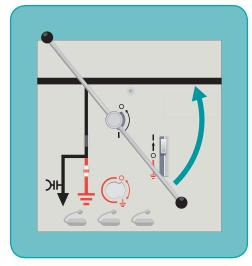
2 Insert the operating lever and rotate anti-clockwise to open the Isolator Switch.
