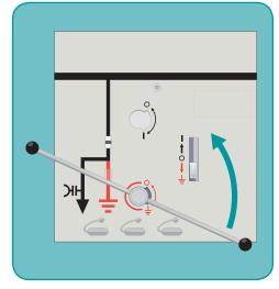
Insert the Operating Lever and rotate 2 Insert the Operating Level and College anti-clockwise to open the Earth Switch.
