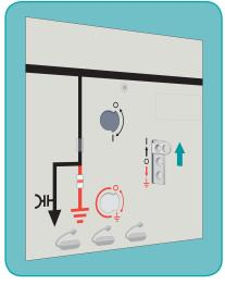
Slide the Control Gate up to open the Isolator Shutter.
