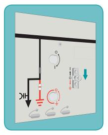
Remove the Operating Lever. Check the Control Gate has returned to the mid position.
