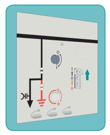
Slide the Control Gate up to open the Isolator Shutter.
