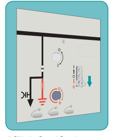
Slide the Control Gate down to open the Earth Shutter.
