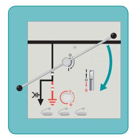
2 Insert the Operating Level and Colockwise to close the Isolator Switch. Insert the Operating Lever and rotate
