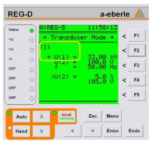
In the transducer mode you can see both voltages, the frequency and the supervision limit for the unregulated voltage.
