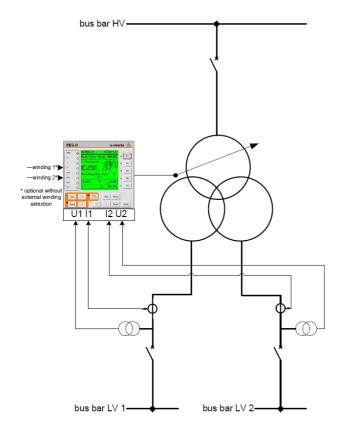
A three winding transformer is a power transformer that has two secondary windings that normally feed different bus bars. The voltage on the secondary windings can be equal or different. Normally the transformer has only one OLTC on the primary side so that it is necessary to connect both secondary voltages to the regulator to allow selection of either one for regulation as appropriate.
