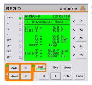
On the second transducer screen you can find the current, phase angle and the power of the regulated measurement input.
