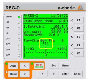
The voltage that is used for regulation is indicated in the regulator screen. The default is a {1} for voltage input 1 and a {2} for voltage input 2. However, in setup this indication can be changed to a user definable 3 character string, e.g. 33k.
