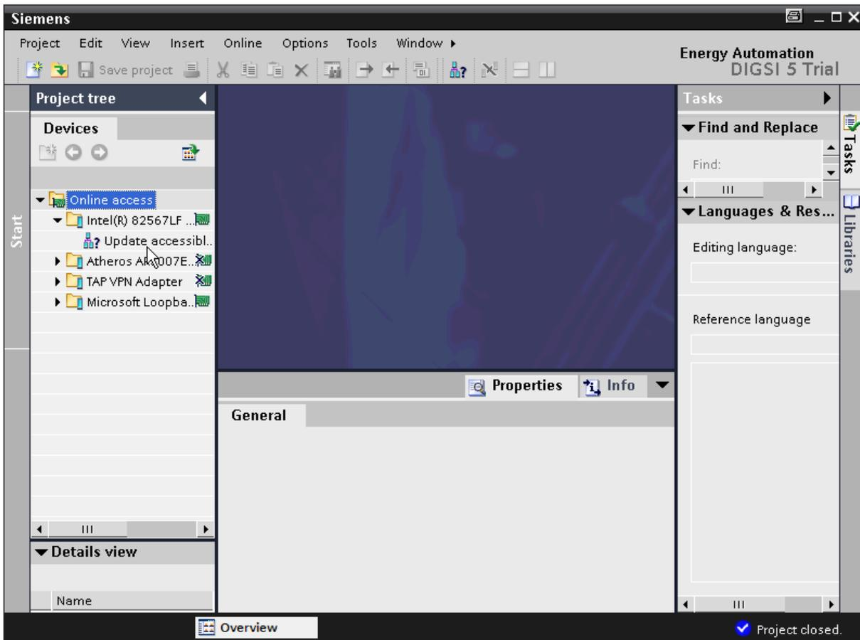
Figure 3: Find accessible devices in DIGSI 5
