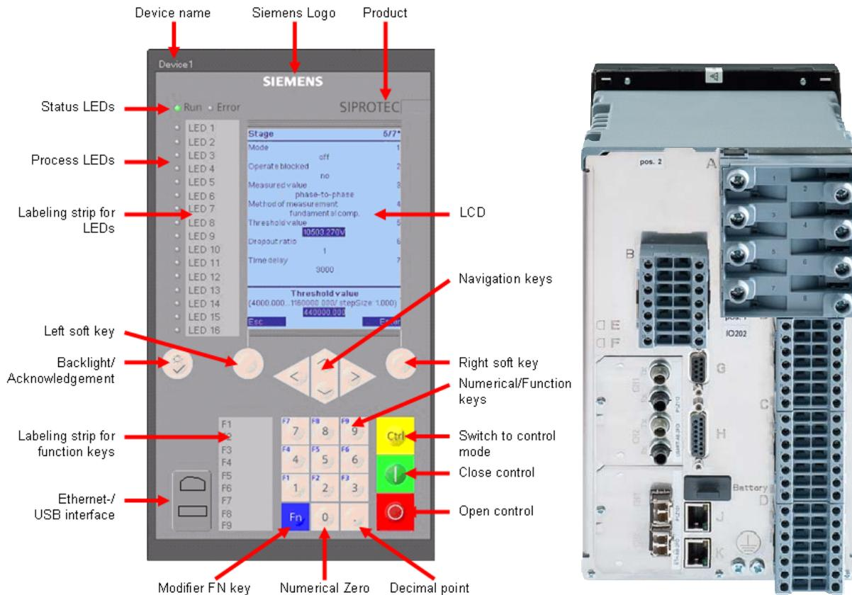
Figure 2: SIPROTEC 5 device front and rear view with optical port E (port J is always electrical)
