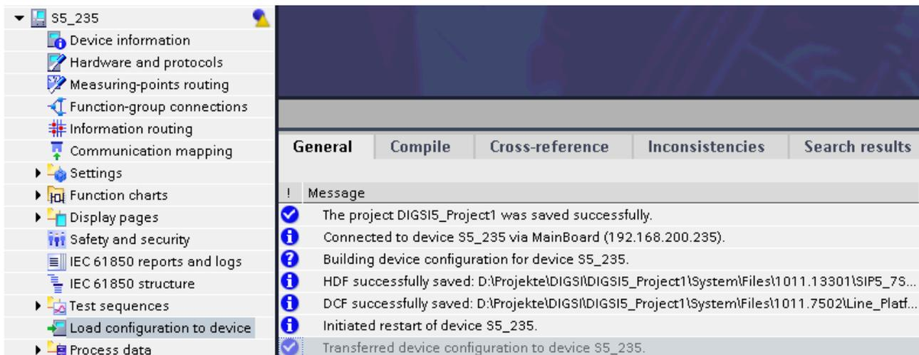
Figure 9: Load configuration to device
