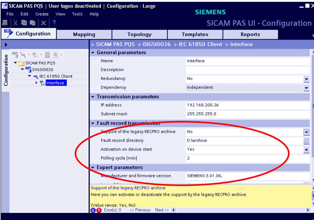
Figure 14: IEC 61850 settings for fault record transmission
