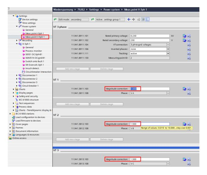
Application for low voltage with 400 V measurement without voltage transformer
