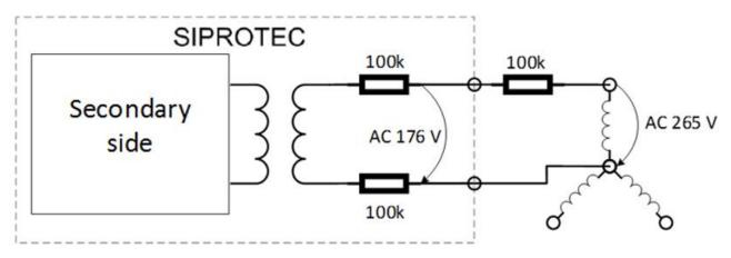
Series connection of an external  $100 \text{ k}\Omega$  resistor divides the low voltage (e.g. 265 V phase-earth = 230 V + 15%) by a factor of 1.5, so that a suitable or permissible voltage is applied to the device terminals (e.g. 176 V = 265 V / 1.5).
