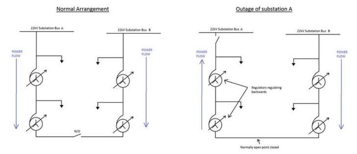
During an outage of Substation A, power must flow in reverse through the two transformers on the left, towards the distribution network. When this happens, the voltage on the Bus A side of the transformers should be monitored instead, and the functioning of the tap changers should be inverted. Achieving this with multiple controllers can be costly and complicated.
