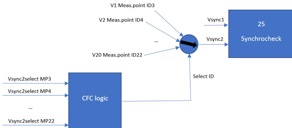
Fig.6: Overview Voltage Selection functionality
