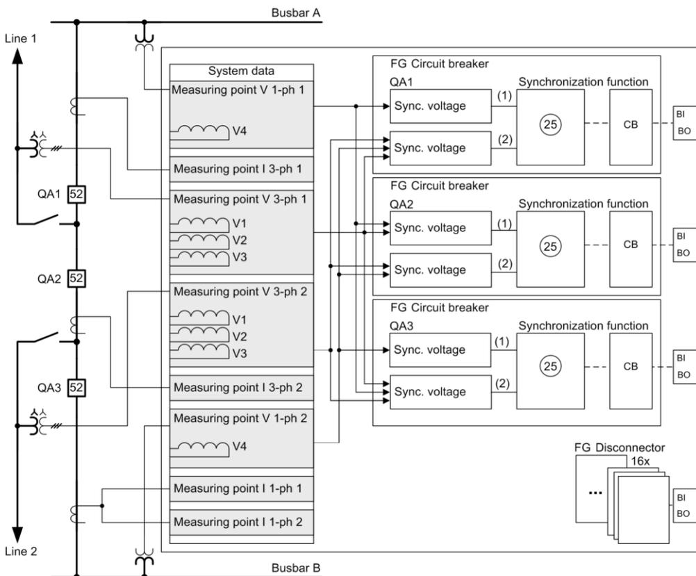
Fig. 1: Synchronization in a Breaker-and-a-half arrangement
