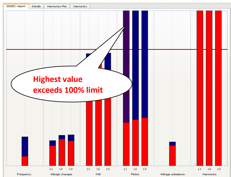
Figure 4. Example of EN 50160 report, where 100 % limit has been exceeded – shown by cross hatch blue graph section (but the 95 th percentile has not exceeded the 95 % limit).
