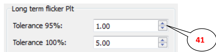
Figure 32. Infraction Flicker long term, limit is set by the narrow setting.
