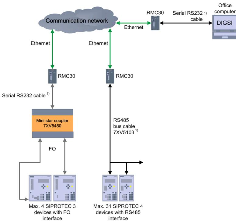
Figure 1: Extended COM Port RS232/485 with RMC30
