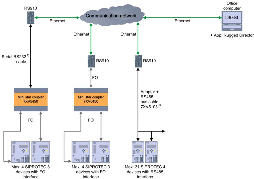
Figure 4: Virtual COM Port for Optical Fiber/RS232/485 with RS910
