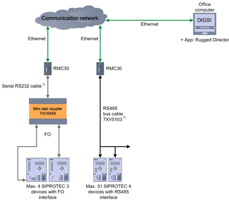
Figure 2: Virtual COM Port RS232/485 with RMC30
