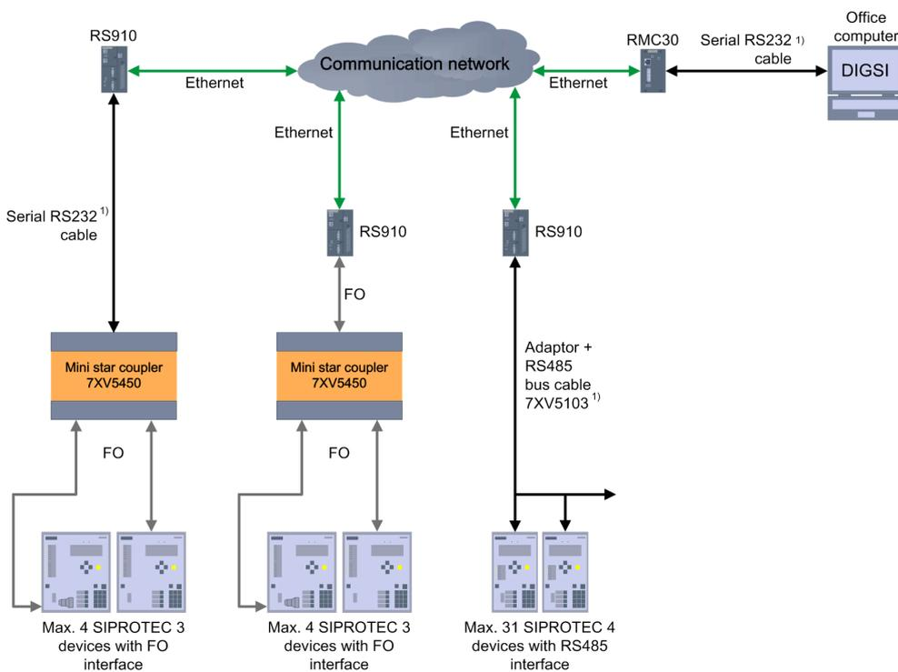
Figure 3: Extended COM Port for Optical Fiber/RS232/485 with RS910
