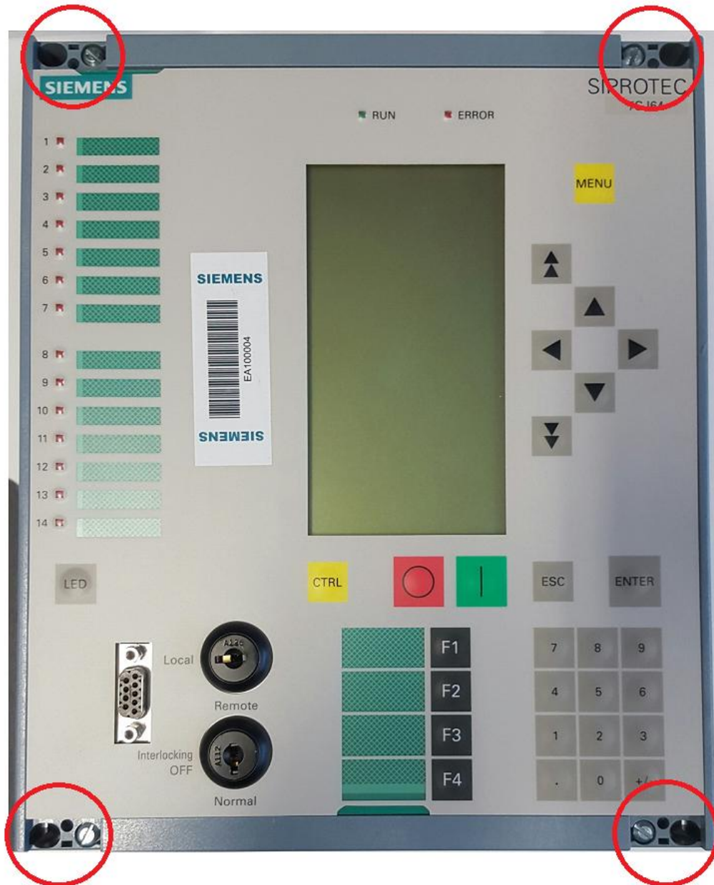
Figure 2: 4 screws holding the faceplate to relay housing
