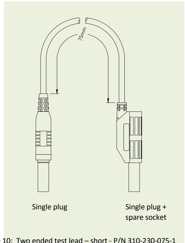
Figure 10: Two ended test lead – short - P/N 310-230-075-1
