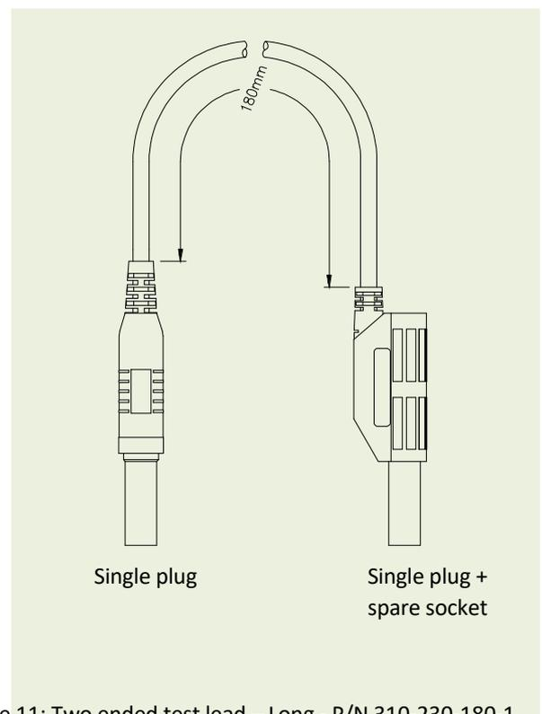
Figure 11: Two ended test lead – Long - P/N 310-230-180-1
