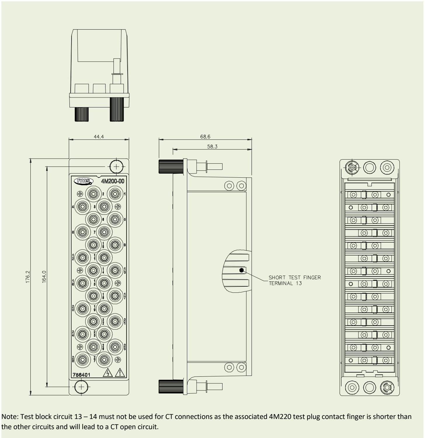
Note: Test block circuit 13 – 14 must not be used for CT connections as the associated 4M220 test plug contact finger is shorter than the other circuits and will lead to a CT open circuit.
