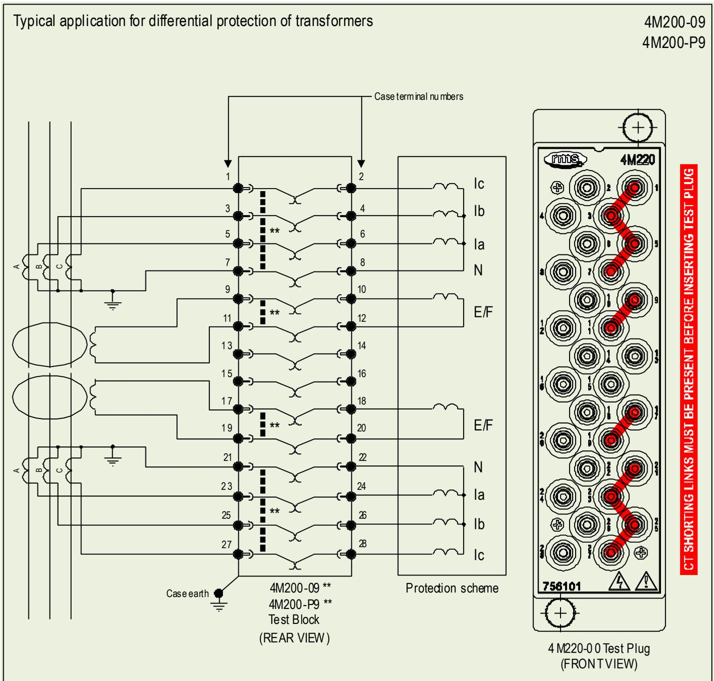
Figure 7: Typical application for differential protection of transformers
